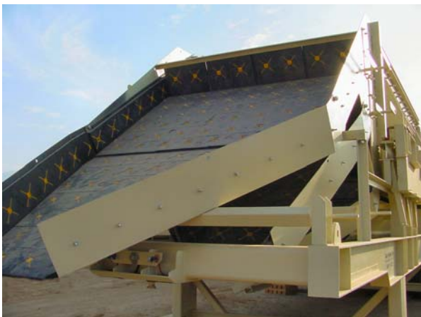
Three discharge chutes with blending gates on the top two decks to provide separate or mixed products. (shown with urethane liners).
